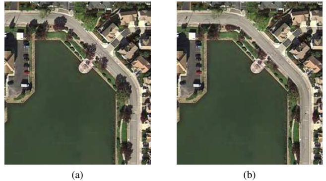
Fig. 2: An example of the shadow removing preprocessing, (a) original satellite image, (b) processed image.
