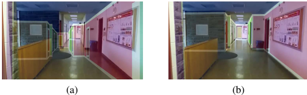
Figure 6: An example of the ground-truth labeling process: first roughly estimate the camera pose, and overlay its view in the 3D floor-plan with the actual image, as shown in (a). Then change the 6-DoF camera pose with an interactive interface, until the two views are consistent as shown in (b).
