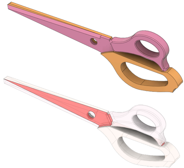
Figure 15. Two bodies (top) and their respective contacts highlighted in red (bottom).
